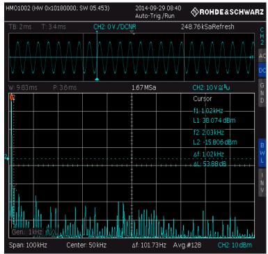
Vertical is the sound level, horizontal the audio bandwidth (0-100kHz). At left is our 1kHz test signal.
