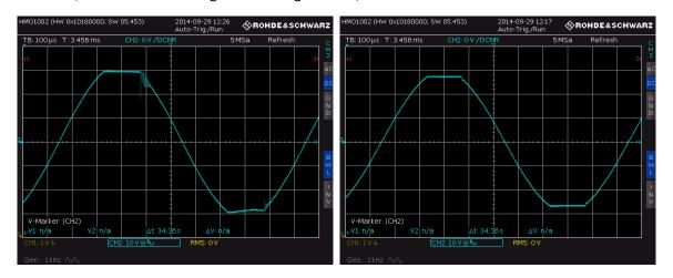
At left: Hexfets tend to show only some minor and harmless high frequency oscillation when driven into clipping as visible just after the positive and negative tops.
