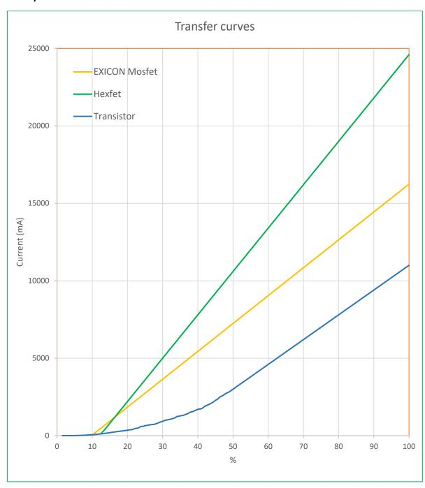
Horizontal represents the % of conductance, vertical the current of the output stage.
