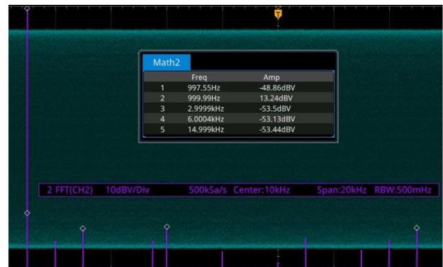
Frequency domain (50kHz wide). Harmonics < 65dB (13+53). The irritating 3<sup>rd</sup> harmonics (3kHz) is at this low level. Even more irritating 5<sup>th</sup> is below the scale actually.
