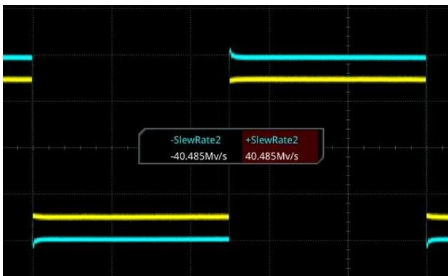
1kHz square wave signal without any significant irregularities like swing in/out. It also shows a slew rate of around 40V/uS. Please note that high quality opamps hardly reach 12V/uS...
