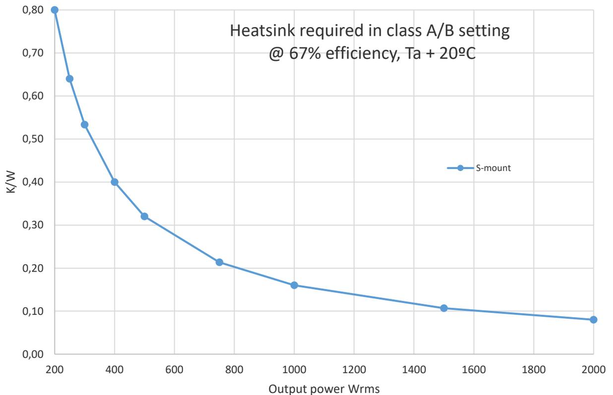
*Note that the max. output power strongly depends on the supply voltages, type of Mosfets used and the dissipation rate (K/W) of the heatsinks mounted.*
