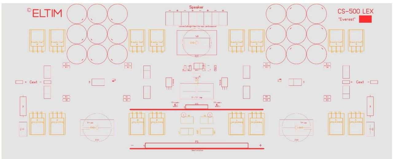
CS-500 layout with eight pairs of EXICON Mosfets at the back side, positioned in a way that there is a maximum heat transfer to the immense heatsinks of a MODU Dissipante 435x500x210mm cabinet where it actually just fits.
