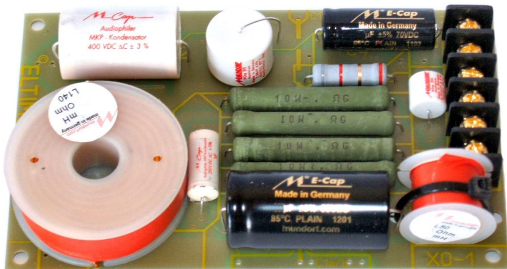
This XO-1 PCB fits about all kinds of wire/foil coils, capacitors and resistors.
