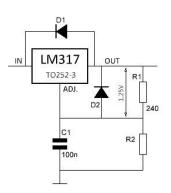
Champion in regulating behaviour, are the <u>LM317</u> (pos.) and <u>LM337</u> (neg.) voltage regulator IC's, capable of delivering up to 1500mA. In the replacement modules we present here, we use small SMD TO252-3 types. Unlike 78xx/79xx they can be "programmed" by the values of two resistors. Since R1 is of a fixed value, the value of R2 defines the output voltage. A capacitor C1 is added for better behaviour, less noise, etc.
