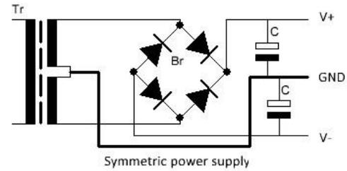
Then, just by relocating the ground connection to a centre tab on the transformer, we obtain a symmetric supply voltage, meaning a V+ (higher than ground) and a V- (lower than ground) voltage. With same voltage secondary windings, this ground level is exactly between V+ and V- or in other words, V- has the same voltage as V+ except for reversed polarity.
