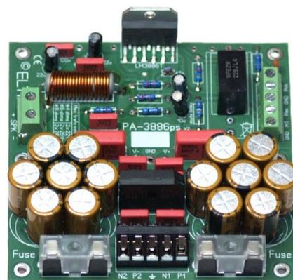
100x100mm, 80W amplifier module with integrated symmetric power supply using audio grade NICHICON ‘Fine Gold’ supply capacitors
