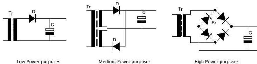
In the very early tube days, only the most left schematics was used where the diode was a rectifying tube. Only a half sine is rectified and charging the storage capacitor, causing quite some hum. The transformer is only loaded on the positive sines, so used very inefficiently.
